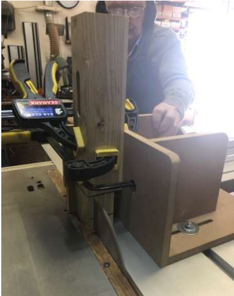
Cutting tenons on table saw
