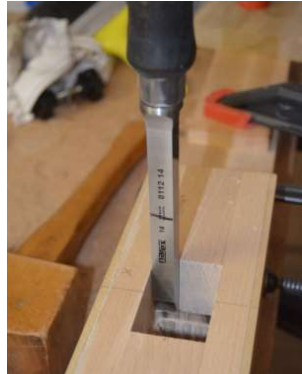
Trimming with a mortise chisel aligned by a jig
